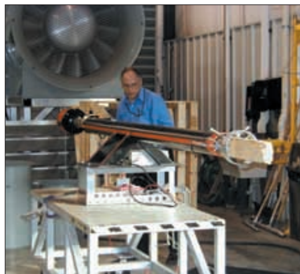
Large missile impact test on a model USGF fan.
