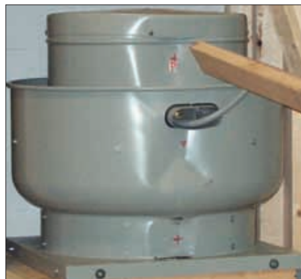
Large missile impact test on a model USGF fan.
